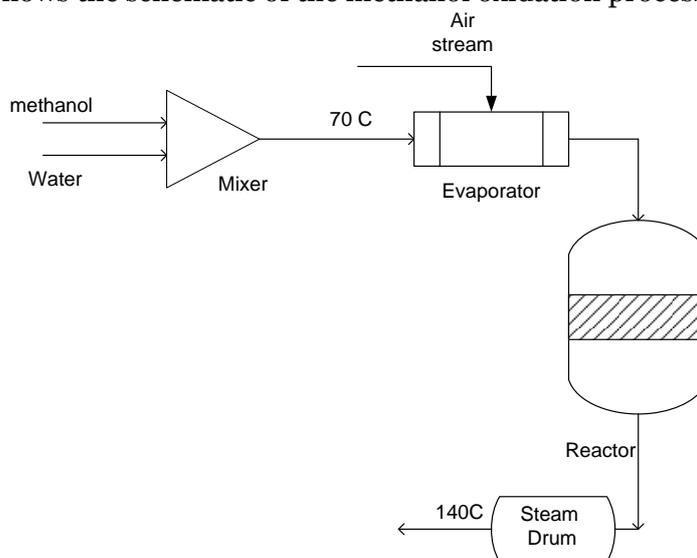
Figure 1. Oxidation of methanol process
