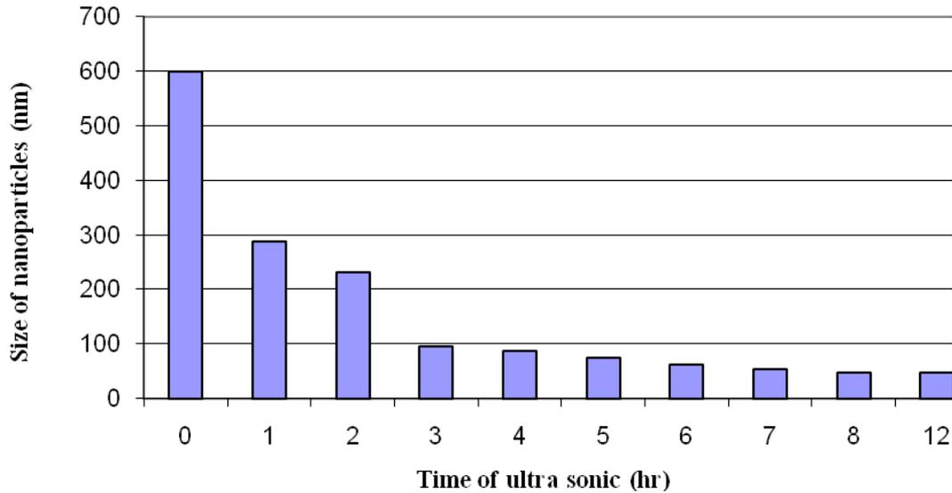
Figure 1. Size of particle versus time of ultrasonic.
