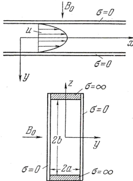
Figure 1. Diagram of flow of water in the MHD-cell:  $\sigma$  – conductivity of the cell wall;  $B_0$  – amplitude value of the magnetic field induction vector
